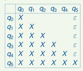
Algorithm A.55: 2. If  $(\delta(p, a), \delta(q, a))$  marked by  $\varepsilon$ , then mark (p, q) by *a* (not applicable)
