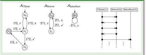
Client-server interaction to get access to an interface. Accepting state is  $(s_3, t_0, q_0)$ .
