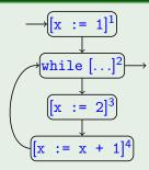
Transfer functions (for  $\delta(\mathbf{x}) = J$ ):  $\varphi_1(J) = [1, 1]$   $\varphi_2(J) = J$   $\varphi_3(J) = [2, 2]$   $\varphi_4(\emptyset) = \emptyset$  $\varphi_4([x_1, x_2]) = [x_1 + 1, x_2 + 1]$
