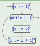
Transfer functions (for  $\delta(\mathbf{x}) = J$ ):  $\varphi_1(J) = [1, 1]$   $\varphi_2(J) = J$   $\varphi_3(J) = [2, 2]$   $\varphi_4(\emptyset) = \emptyset$  $\varphi_4([x_1, x_2]) = [x_1 + 1, x_2 + 1]$
