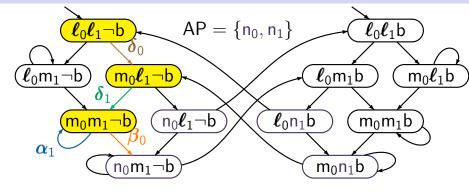
$$\begin{split} \text{ample}(\boldsymbol{\ell}_0\boldsymbol{\ell}_1\neg b) &= \; \{\boldsymbol{\delta}_0\}, \quad \text{ample}(m_0\boldsymbol{\ell}_1\neg b) = \{\boldsymbol{\delta}_1\} \\ \text{ample}(m_0m_1\neg b) &= \; \{\boldsymbol{\alpha}_1, \boldsymbol{\beta}_0\} \end{split}$$
